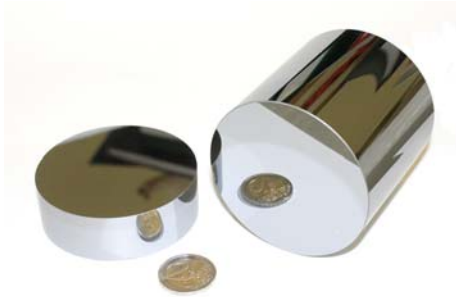
Fig.1 - Two different samples with a diameter of 3'' that are used to investigate the mechanical Q-factor.
