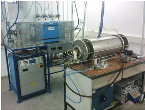
Fig. 1: This picture shows the installed 3-Zone-Furnace and the High-Temperature-Furnace.
