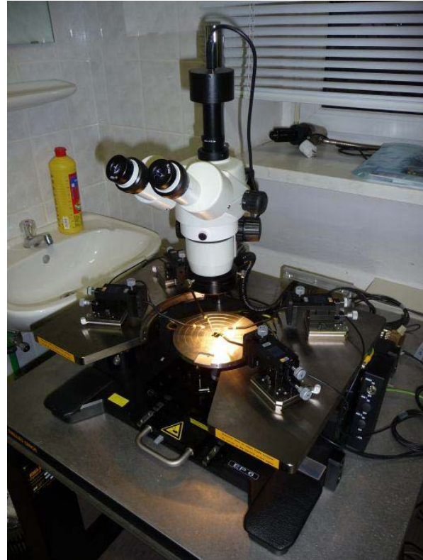
Fig. 1: Süss EP6 DC probe station with stereo microscope (magnification: 15x-100x, fiber optical light ring, 1,3MPixel USB-CCD-camera).
