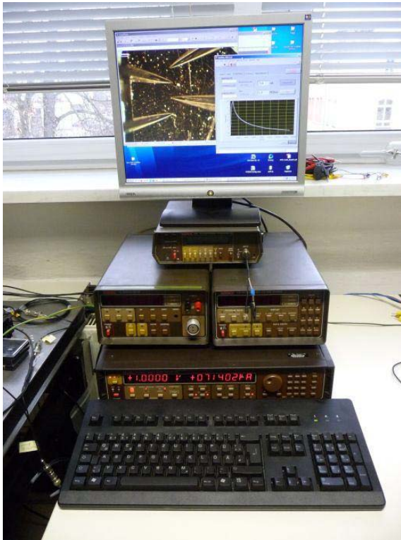
Fig. 2: Electrical measurement setup consisting of source-measure-unit, nanovoltmeter, programmable voltage source and picoammeter. All devices can be controlled with Labview via the IEEE-interface.
