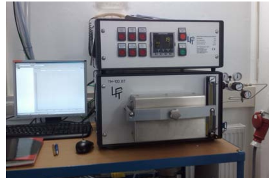
Fig. 1: The RTP sintering furnace TM100BT: In the lower part the reaction chamber and the gas flow controller, in the upper part the Eurotherm is arranged.
