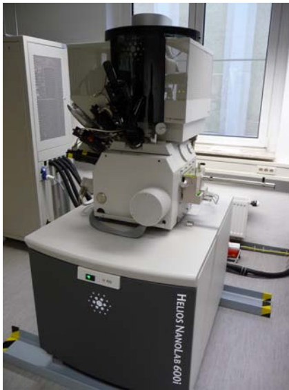
Fig. 1: Photograph of the focused ion beam system (FIB) FEI NanoLab Helios 600i.
